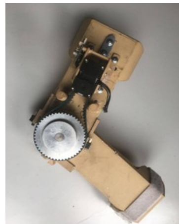
Fig. 2. Prototype of the orthosis with actuator and a reduction gear
