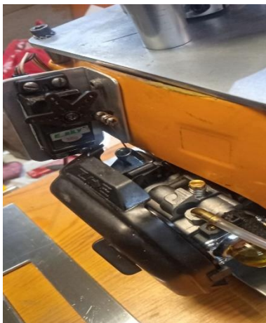
Figure 2. ICE throttle control
