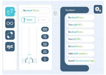
Fig. 8 Determining direction and step length in Photon Code (Master Level)
