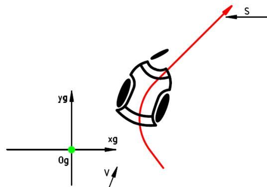
Fig. 1.2 Position of the robot and the set trajectory in the horizontal plane of movement
